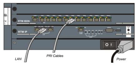
7 E1 or 9 T1 cables can be connected to each RTM ISDN card, up to a total of 14 E1 or 18 T1 PRI cables when two RTM ISDN cards are installed.
